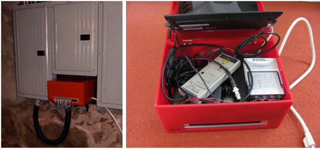
Figure 5: The REDDBox, installed in a home (left) and showing internals (right).
